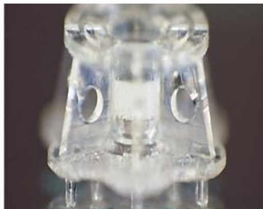
3D-printed gas diffusion layer for an electrochemical reactor, printed at the Cornell NanoScale Science and Technology Facility using two-photon polymerization. Sobhani Lab/Provided
