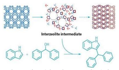
monitoring the formation of ITIs. The researchers tried out the ITIs as catalysts in three popular acid-catalyzed reactions, including a Friedel-Crafts alkylation, a Claisen-Schmidt condensation, and polystyrene cracking. Overall, the turnover rate of the new catalysts was up to six times as fast as commercial zeolites. Source : Chemical & Engineering News, 3/21/2022.
