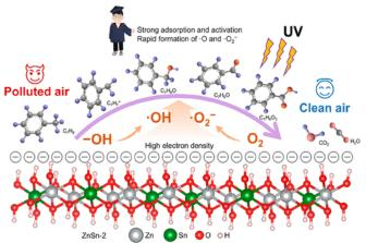
and  $\bullet O^{2-}$ , which allowed rapid opening of the aromatic ring and deep oxidizing into CO<sub>2</sub>. 100% of toluene removal and mineralization efficiency was attained on ZnSn LDH at a high weight hourly space velocity (WHSV) of 60 000 mL gcat<sup>-1</sup> h<sup>-1</sup>. Source: ACS Catal. 2023, 13, XXX, 5529–5537
