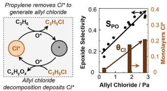
times in flow reactors as well as transient, low-conversion batch epoxidation reveal allyl chloride, formed via propylene oxychlorination, to be a highly unstable intermediate.
