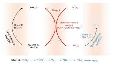
spontaneous redox reaction, electrochemical reduction and electrocatalytic reduction to overcome this issue. RuxCoy alloys were designed and adopted as model catalysts. Ru15Co85
